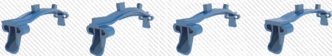
3. -3221 There are 2 track studs per bar with an additional grip bar welded to the underside of the track bar for extreme grip. Only to be used on Nokian Forest King F2.
